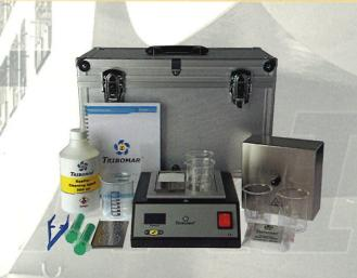
The TriboAmix device is designed to evaluate the compatibility and stability of different and single fuels.
